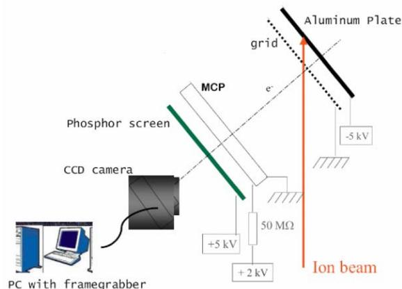
Figure 2: Low intensity beam profiler.
