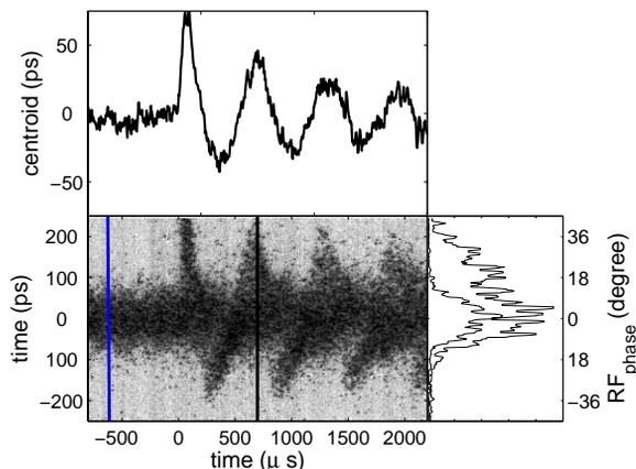
Figure 1: Streak camera image showing the beam at injection. The energy and phase are mismatched at injection. The top figure shows the centroid of the beam distribution, which oscillates at the synchrotron frequency ( $f_S \approx 1.6$  kHz). The right-hand side graph shows the electron bunch distributions at  $610 \mu\text{s}$  before the injection and  $700 \mu\text{s}$  after injection.
