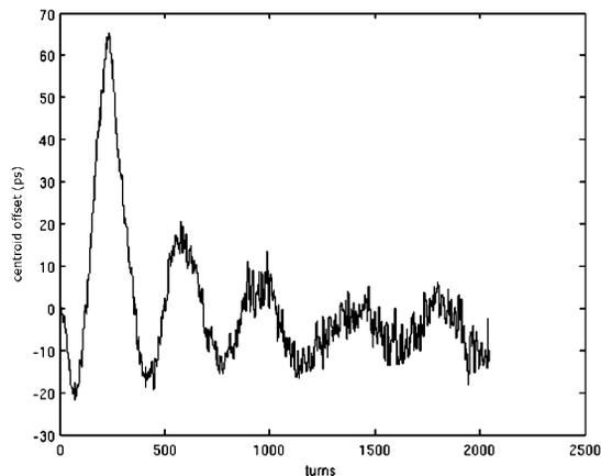
Figure 3: Beam longitudinal phase oscillation at  $1.4 \text{ kHz}$  measured with the phase of the complex signal from the EBPMs.
