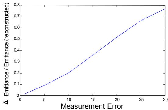
Figure 4: Measurement error vs. projected emittance
