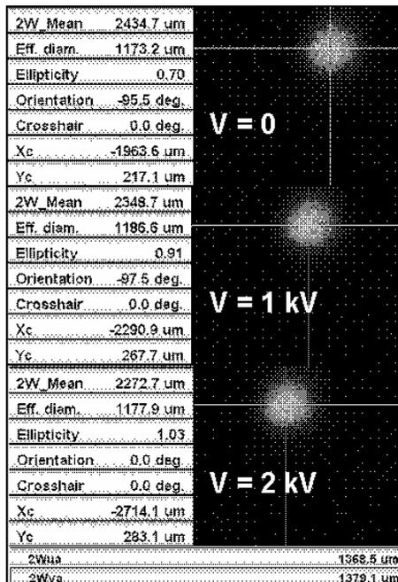
Figure 4: Beam scanning with input diameter of 2mm. Total shift was 75  $\mu$ m with a waist of 68  $\mu$ m.
