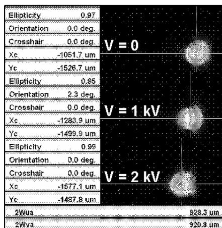
Figure 5: Beam scanning with input diameter of 3mm. Total shift was 52  $\mu\text{m}$  with a waist 46  $\mu\text{m}$ .
