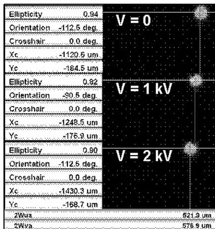
Figure 6: Beam scanning with input diameter of 2mm and beam expander after EO prism. Total shift was 31 $\mu\text{m}$  for 26  $\mu\text{m}$  waist.
