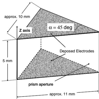
Figure 2: 3D sketch of EO prism. The grey surfaces are metallic coated.
