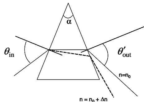
Figure 1: Electro-optic prism. The dashed line represents the beam path when the refractive index is changed.
