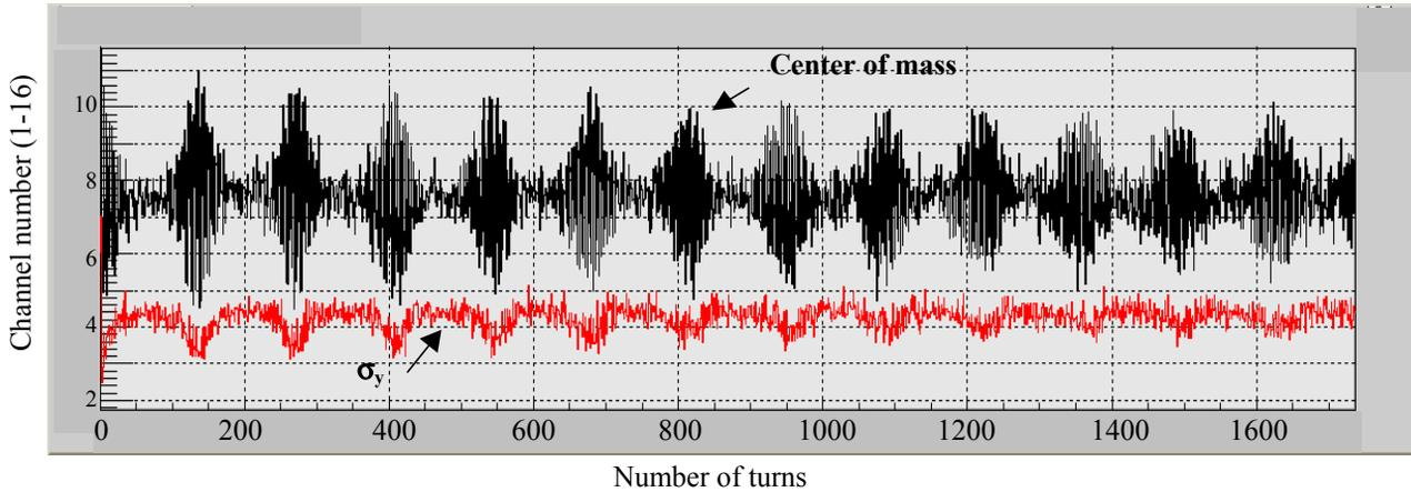
Figure 3: Beam dipole y-oscillations (upper plot) and  $\sigma_y$  behavior (down plot) after a short kick. Duration of the single turn is 1220 ns. Channel constant is 0.12 mm.  $I_{e^-} = 20 \mu$ A.  $C_y = 20$ .  $E = 1843$  MeV.
