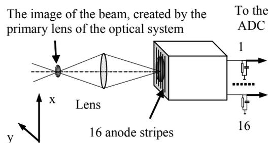
Figure 2: Optical layout of the diagnostics.
