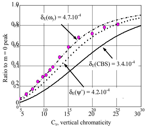
Figure 5: Ratio of  $R_1/R_0$  for different energy spread  $\delta_E$ . Experimental points for  $E = 1843$  MeV are shown.
