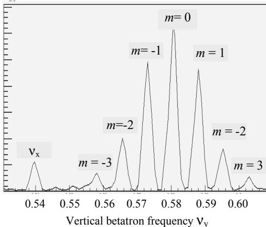
Figure 4: A spectrum of vertical betatron oscillations.
