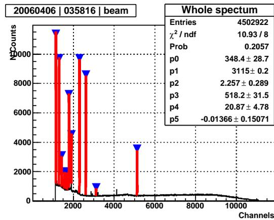
Figure 3: Experimental spectrum of backscattered photons with calibration lines
