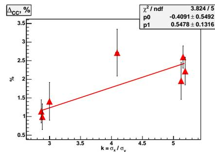
Figure 5: Measured dependence of the jump in the Touschek particle counting rate on the ratio of the horizontal and vertical beam sizes.
