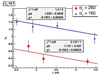
Figure 4: Dependence of the jump in a total counting rate of two counters (without detachment of background) on the bunch current at two values of the vertical beam sizes (given in a.u.).
