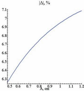
Figure 1: Jump vs. the counter position at  $E=1840$  MeV,  $\zeta = 80\%$  in the 1D approximation.
