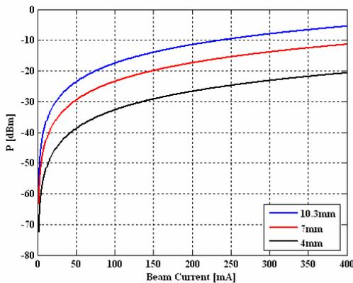
Figure 3: Button delivered power vs. beam current.
