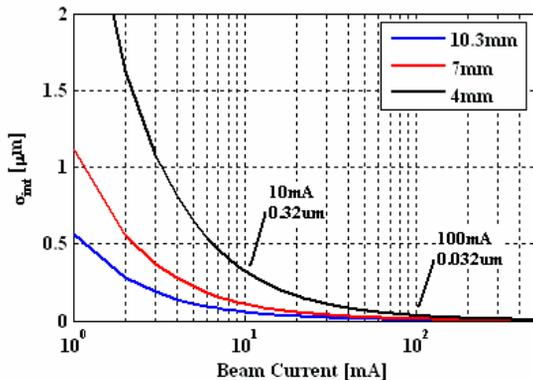
Figure 4: Intrinsic resolution vs. beam current @ 4kHz.
