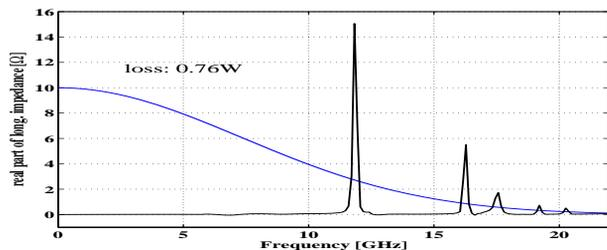
Figure 6: Coverage of the bunch spectrum (bunch length 4.6mm) with the real part of the longitudinal impedance of the chosen BPM.
