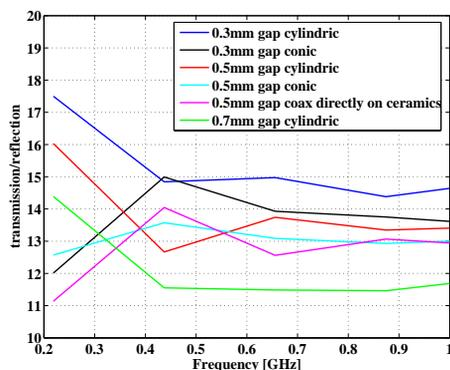
Figure 5: Ratio of transmission to reflection of different buttons. The one of 0.3mm gap and cylindrical form has the best ratio at 500MHz.
