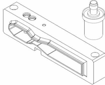
Figure 1: SR BPM block and button pickup.
