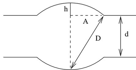
Figure 1: Schematic layout of a confocal resonator [1].
