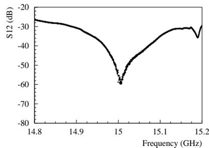
Figure 6: Same as Figure 5, but there is no coupling iris between the waveguide and the nearly-confocal resonator.
