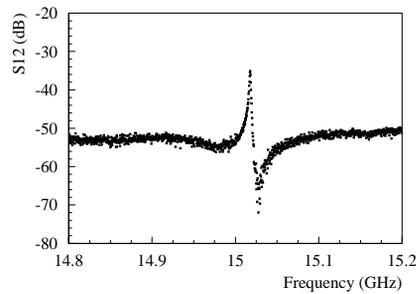
Figure 5:  $S_{12}$  parameter versus frequency for a nearly-confocal resonator installed on a pipe and under-critically coupled to a waveguide through a small iris. The input port is a microwave horn at one end of the pipe and the output port is the coaxial transition to the waveguide.
