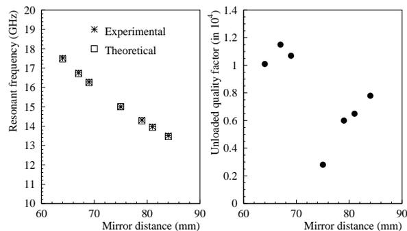
Figure 3: Resonant frequency (left) and unloaded quality factor (right), as a function of the distance between the spherical mirrors of the open resonator prototype.
