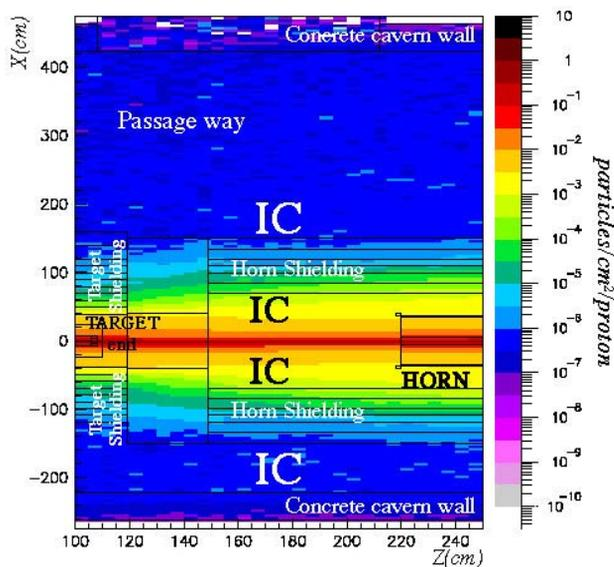
Figure 5: Fluence of all charged particles in the area intended for the ionization chambers location (IC).
