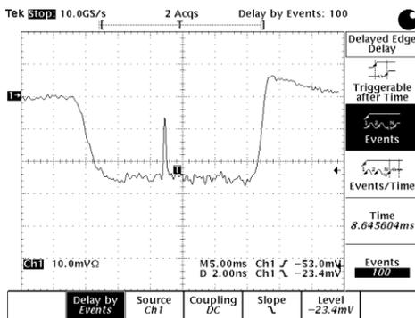
Figure 5: The 100<sup>th</sup> turn of the gating signal with a captured single-shot signal
