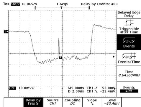
Figure 6: The 400<sup>th</sup> turn of the gating signal with a captured single-shot signal
