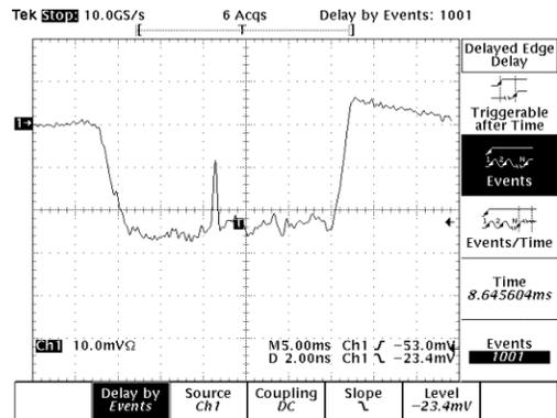
Figure 7: The 1001<sup>st</sup> turn of the gating signal with a captured single-shot signal.
