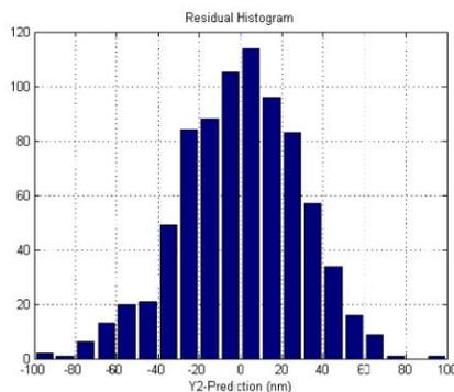
Figure 4: The residuals for 800 ATF extractions from a period spanning roughly 9 minutes on 27 May 2005. The standard deviation of the distribution was 29.4 nm and yielded a resolution of 24.0 nm.
