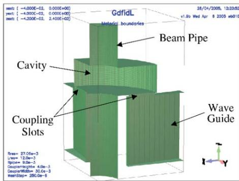
Figure 1: A quarter view of the inside surface of a BINP BPM.
