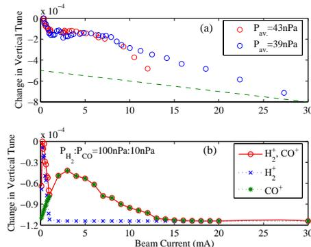
Figure 5: (Upper) (a) Experimental results of change in vertical tune in single-bunch condition in UVSOR-II in different vacuum pressure conditions. Broken line corresponds to the estimation of the wake field effect. (Lower) (b) Tracking calculation of change in vertical tune in single-bunch condition from  $H_2^+$  and  $CO^+$  ions.
