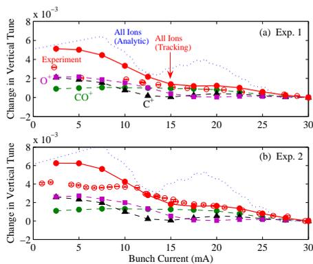
Figure 4: Experimental results (red empty circles), tracking results (filled marks) and analytic calculations (blue broken curve) of change in vertical tune for (upper) (a) Exp.1 and (lower) (b) Exp.2.
