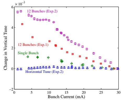
Figure 3: Dependence of tune on beam current in vacuum conditions in Fig. 2.
