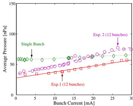
Figure 2: Averaged vacuum pressure for Exp.1, Exp.2 and single-bunch condition.
