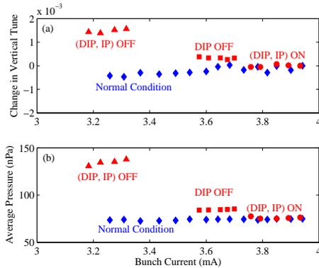
Figure 1: (Upper) (a) Change in the vertical tune when vacuum pumps were intentionally turned off (red marks) and when the normal vacuum condition (blue marks). (Lower) (b) Change in average pressure when the pumps were turned off.
