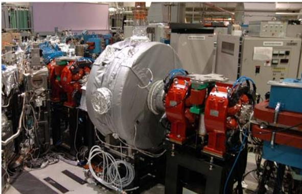
Figure 4: Photograph of new cavity covered with jacket heaters. A view from outside the storage ring.
