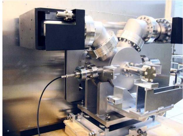
Figure 1: Gun with the ion pumps.
