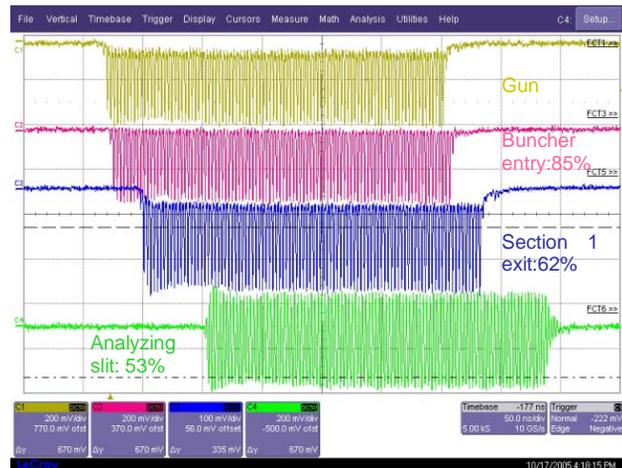
Figure 2: Beam transmission for the LPM mode.
