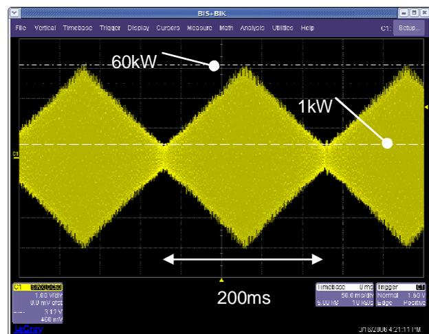
Figure 4: Oscilloscope trace of 5Hz fast ramping of power in booster cavity.
