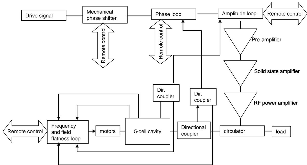
Figure 2: Interfaces between components in the booster RF system.
