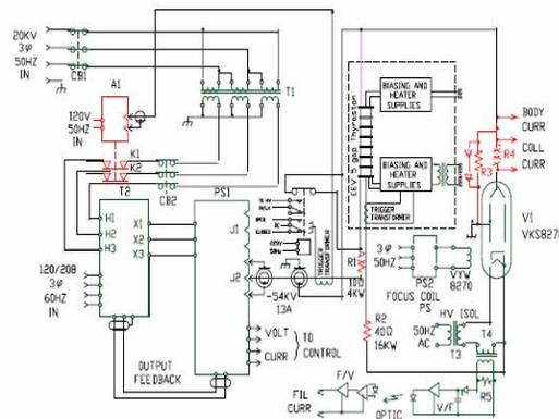
Figure 6: A schematic of the HVAC and crowbar operation of the high power RF system.
