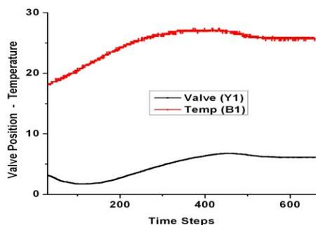
Figure 4: Operation of the cooling controller for the wave-guiding subsystem: The sensed temperature is the input signal (B1) to the controller; the generated analogue output signal (Y1) is directly connected to the mixing valve actuator. The requested temperature (set point) in this case is 26° C.
