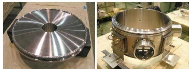
Figure 1: Second test cavity, made of steel (SS400), to examine the vacuum performance of the new copper electroplating. The endcap (left) and barrel (right) parts.
