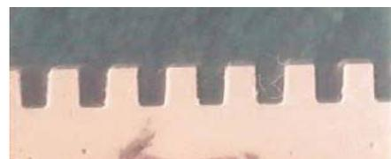
Figure 7: Replica of the grooves of the outer conductor of the coaxial line for the first prototype.
