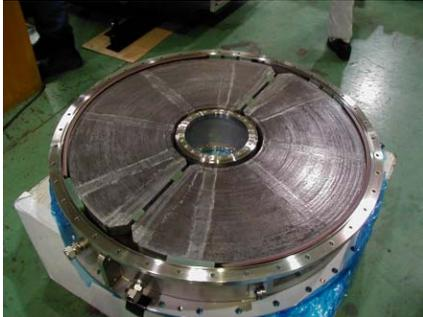
Figure 7: MA core without coating.
