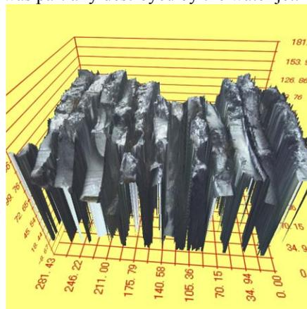
Figure 1: Three-dimensional microscopic view of the surface by water jet. Each ribbon was split and removed by high-pressure water.
