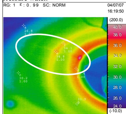
Figure 2: An infrared camera measured the MA core temperature. A white circle indicates the cut core gap. Hot spots were observed.
