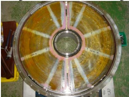
Figure 8: MA core without coating after high power test. The core was used from 2003 on and tested for about 800 hours, in total.
