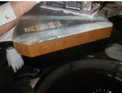
Figure 9: Cut surface after a few 10 hours high power test. The surfaces were not covered by coating and the dissolved oxygen was not controlled.
