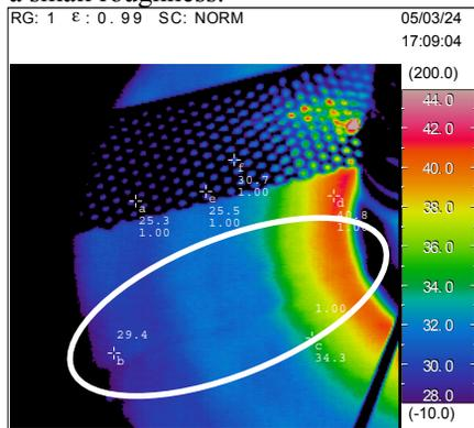
Figure 4: MA core temperature. The cut core gap is surrounded by a white circle. No hot spot was observed.
