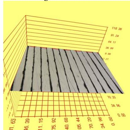
Figure 5: 3D-microscopic view of a “Diamond Polished” surface. The flatness is better than by other methods.
