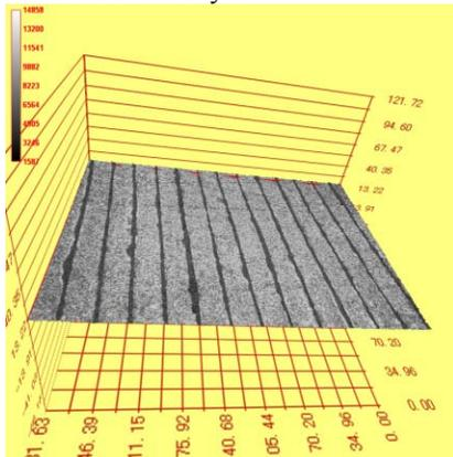
Figure 3: 3D-microscopic view of the surface made by grind stone cutting. The MA ribbons are clearly separated by silica and epoxy resin. Thanks to etching, the surface has only a small roughness.
