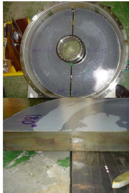
Figure 10: MA cores using Diamond Polishing. 98% of the core surface is covered by epoxy coating (top). After 300 hours high power test, the corrosion on cut surface (bottom) is restricted.
