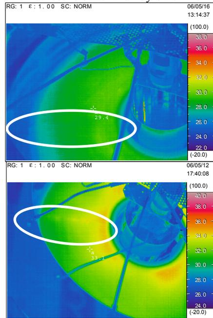
Figure 6: MA core surface temperature. The cut core gap is surrounded by white circles. Two of 6 cores did not show hot spots (top). Others showed hot spots (bottom).
