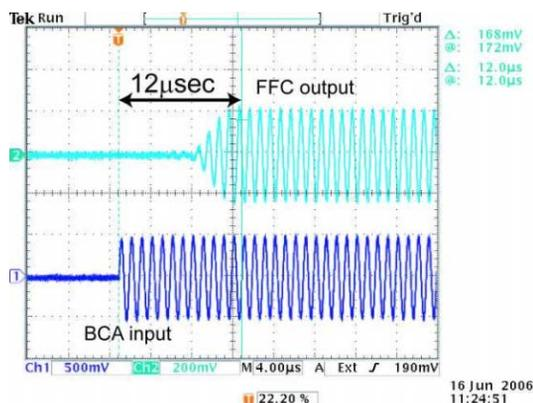
Figure 4: Group delay of the compensation system.
