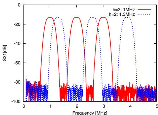
Figure 5: Frequency responses for the different accelerating frequencies.
