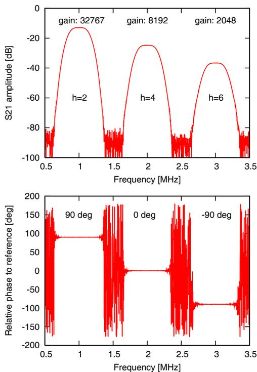
Figure 6: The gain and the phase of each harmonic is set individually.
