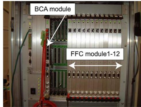
Figure 3: BCA and FFC modules in the 9U VME chassis.
