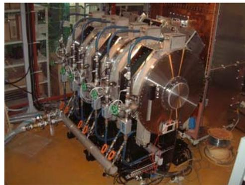
Figure 1: The MA cavity for the RCS.
