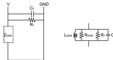
Figure 3: The one by one measurement of the core.
