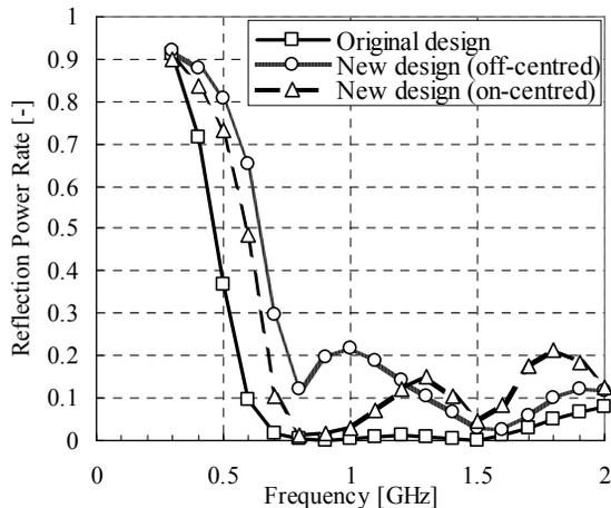
Figure 4: Reflection characteristic of HOM damper for original design and new design by HFSS code
