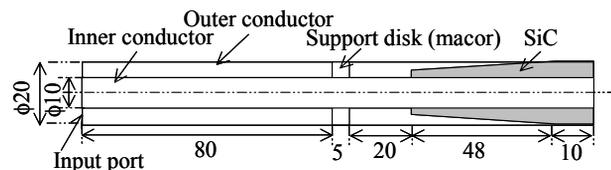
Figure 2: Cross-sectional view of the original HOM damper
