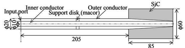
Figure 5: Cross-sectional view of new on-centred damper
