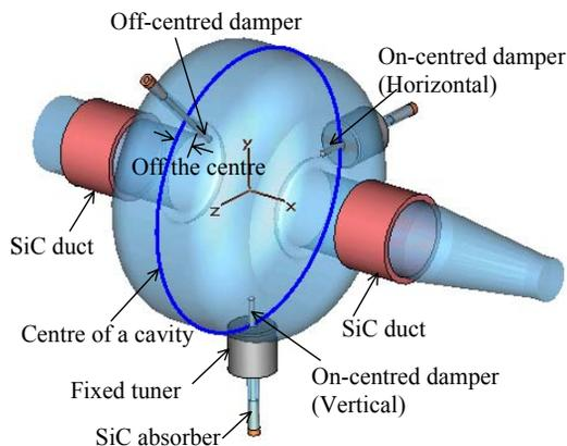
Figure 1: A schematic diagram of a half of the pair cavities with three original dampers
