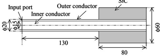
Figure 3: Cross-sectional view of new off-centred damper
