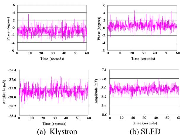
Figure 3: Pulse to pulse phase and amplitude variation during 60seconds in K5 module.
