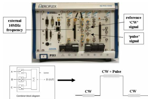
Figure 4: Digital pulse to pulse phase feedback system.
