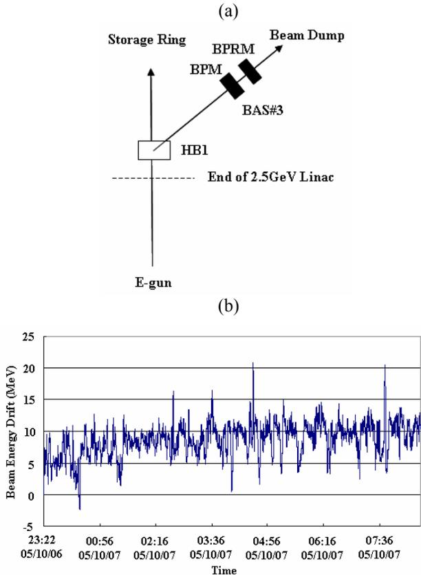
Figure 2: Beam energy drift measurement by BAS#3. BPM (Beam Position Monitor). (a) Beam energy measurement analyzer (b) Results of beam energy drift during 9hours
