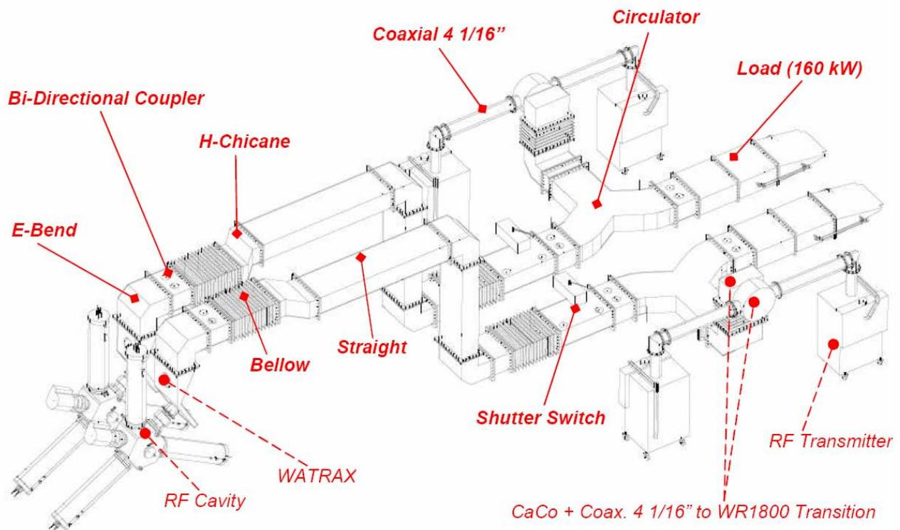
Figure 1: Two RF plants in one straight section.
