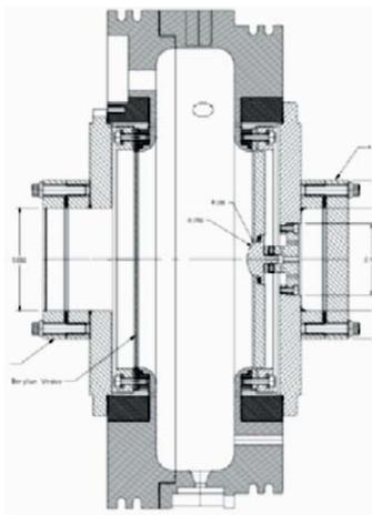
Figure 4: The 805 MHz cavity with a button sample holder on the right and thin windows on the left.
