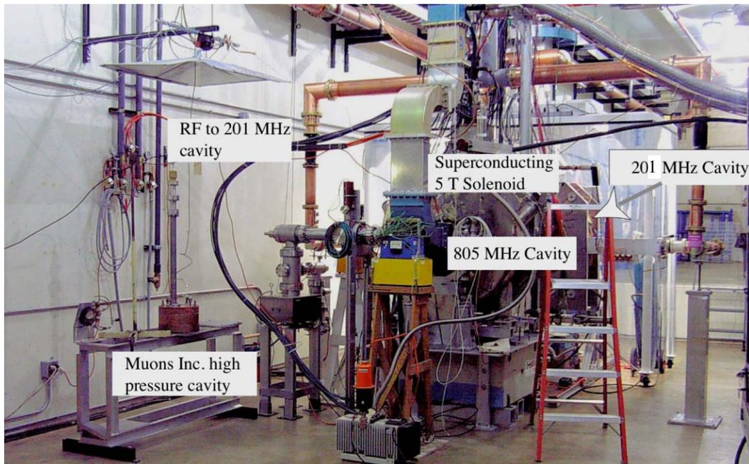
Figure 3: The 805 and 201 MHz cavities and the 5 T solenoid magnet, looking toward the linac where the power supplies are located.
