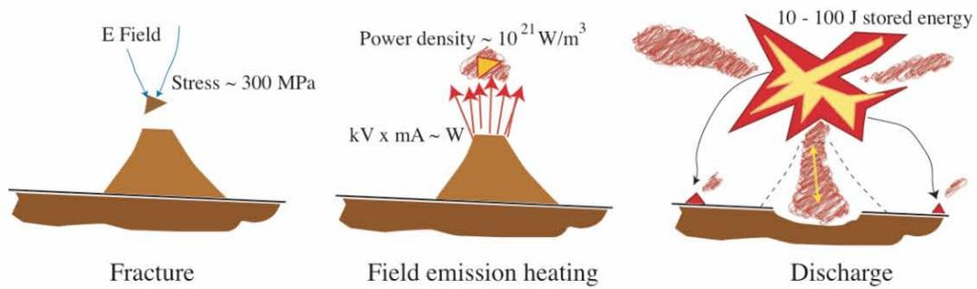
Figure 2: The breakdown model. The initial fracture can be influenced by temperature, magnetic field, material and electric field, the field emission heating stage can be influenced by the gas pressure and type, and the discharge phase is influenced by the stored energy, pulse length, geometry and frequency.
