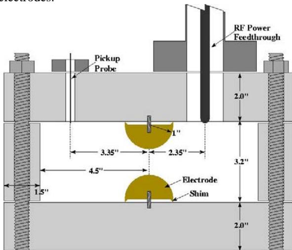
Figure 1: Cross section of the test cell showing the replaceable one inch radius Cu, Mo, or Be hemispherical electrodes. The top and bottom plates and the cylinder are copper-plated stainless steel (the gas input/exhaust port is not shown in the figure).
