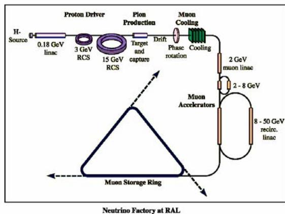
Figure 1: A typical Neutrino Factory schematic
