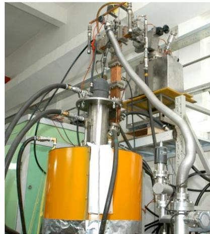
Figure 5: IHEP-made 45MW klystron
