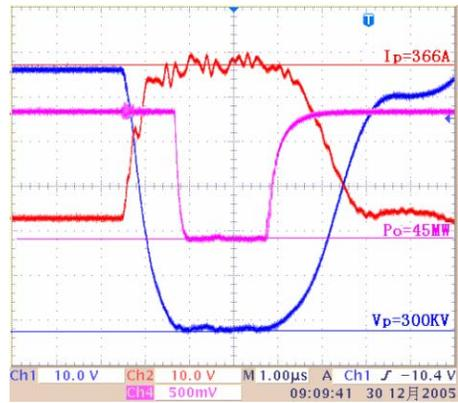
Figure 3: waveform of IHEP-made 45MW klystron
