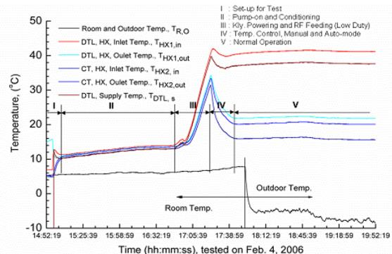
Figure 4: Cooling water temperature variation during operation (DTL cooling system).
