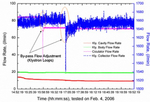
Figure 5: DTL klystron cooling water flow variation during operation.
