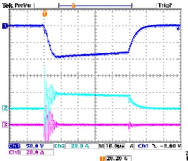
Figure 2: Pulse power using opening switch (horizontal : 10µs/div.).
