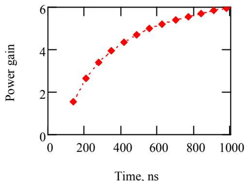
Figure 2: The power gain of the pulse compressor as a function of the input RF pulse length.
