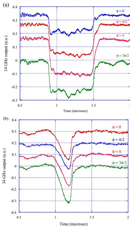
Figure 2. Output power traces showing all four output arms of the magnicon for both long pulse (a) and short pulse (b) operation
