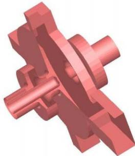
Figure 6. A three dimensional picture of the breakdown cavity is shown which was used to model the cavity and place the maximum electric field on the test stubs.
