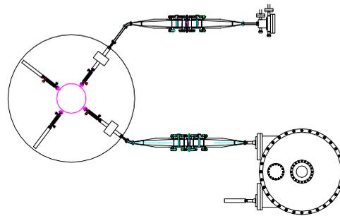
Figure 3. Schematic of Ka-band facility layout showing magnicon on left and two experiments, the pulsed heating at the top and the quasi-optical pulse compressor below.
