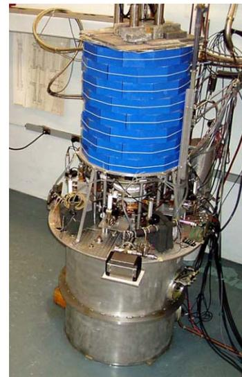
Figure 1. The Yale/Omega-P, 34 GHz magnicon as installed in the Yale Beam Physics Lab
