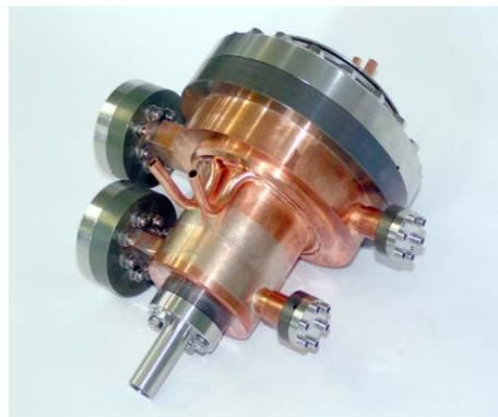
Figure 4. Pictured is the pulsed heating cavity which is awaiting installation onto one arm of the magnicon.
