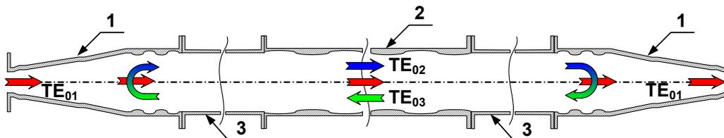
Figure 1: One-channel SLED-II pulse compressor. **1** -  $TE_{02} \leftrightarrow TE_{03}$  reflective mode converter; **2** -  $TE_{01} \rightarrow TE_{02}$  transmission mode converter; **3** - waveguide delay lines.
