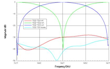
Figure 5: Results of calculation of mode conversions in the  $TE_{01} \leftrightarrow TE_{02}$  mode reflecting converter with the  $TE_{02}$  mode incident.
