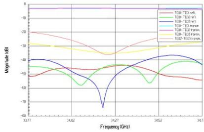
Figure 8: Conversion of the forward  $TE_{01}$  mode into other modes.
