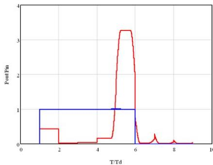
Figure 9: Calculated envelope of the input (blue) and output (red) pulses for the one-channel SLED-II with phase reversal switch time of 50 ns.  $T_d = 100$  ns.
