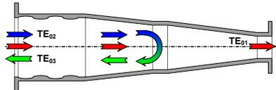
Figure 4:  $TE_{02} \leftrightarrow TE_{03}$  mode converter-reflector.
