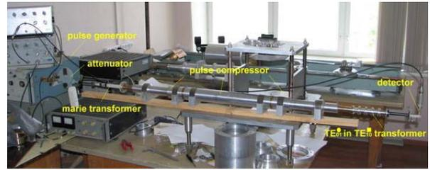
Figure 10. Photograph of the 30 GHz prototype.
