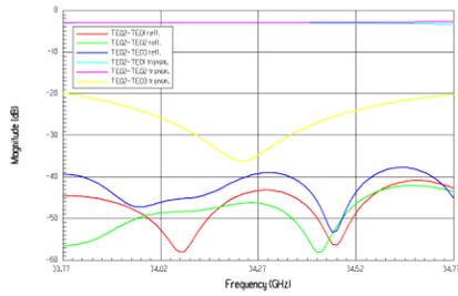
Figure 7: Conversion of the forward  $TE_{02}$  mode into other modes.
