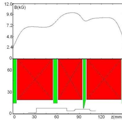
Figure 2a. Magnetic circuit configuration, showing three coils and four iron pole pieces. The plot at top shows the magnetic field profile. The outline drawing at bottom shows the drive cavity (left) and the output cavity (right).
