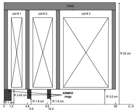
Figure 2b. Schematic design of the room-temperature magnet system. Shown are the dimensions of the three coils, and of the split, removable Armco rings and iron yoke structure. This structure, mounted vertically, is designed to allow removal from the tube without breaking vacuum. The clear bore diameter of 7 cm should be large enough to allow the beam collector to pass through.
