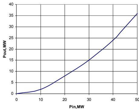
Figure 4. Drive curve, showing output power at 34.272 GHz vs. input power at 11.424 GHz for fixed magnetic field and fixed beam parameters.
