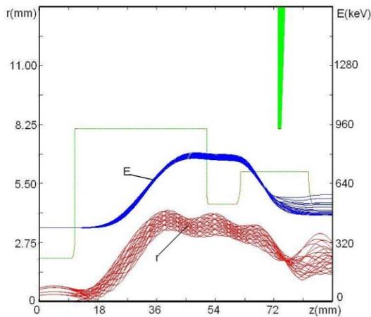
Figure 3. Beam particle energies (blue) and radial excursions (red) for  $n = 3$  (frequency tripler), with the  $TE_{311}$  mode output cavity tuned to 34.272 GHz. Cavity outlines are also shown. Simulations were made using magnicon codes [9].
