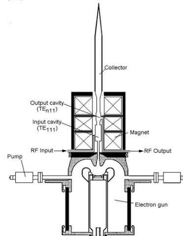
Figure 1. Sketch for conceptual design of harmonic multiplier, not drawn to scale.
