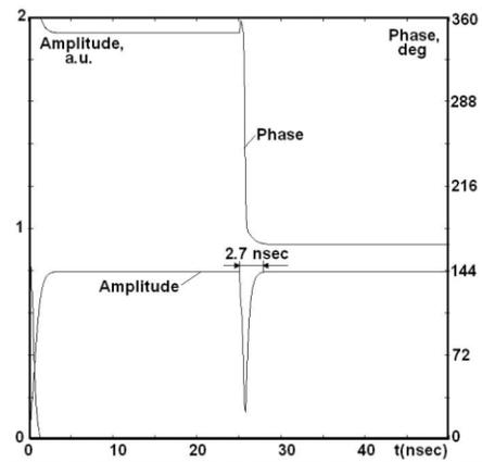
Figure 5. Simulation results for a  $180^\circ$  phase flip in the frequency doubler ( $n=2$ ). Input power is 50 MW. The amplitude and phase of the output signal are shown vs. time. The phase of the multiplier drive signal is assumed to change instantaneously by  $90^\circ$  at  $t = 25$  nsec.
