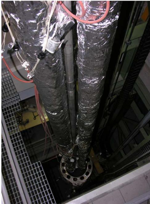
Figure 1: Vertical coating facility. Various cylindrical pipes (5.5m long) are here coated simultaneously. The magnetic coil is visible at the bottom.
