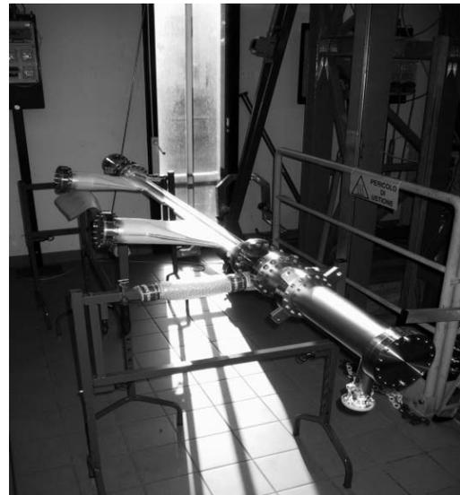
Figure 3: Soleil chamber with lateral pumping ports.
