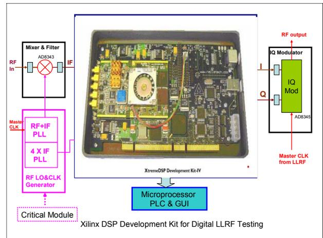
Figure 5: Xilinx DSP development Kit for Digital LLRF System testing.
