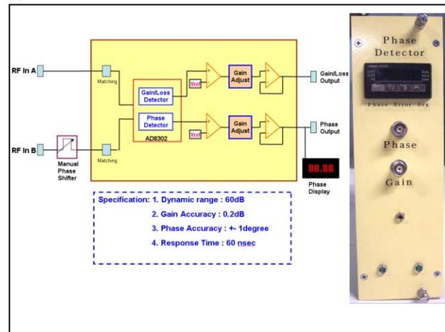
Figure 2: Phase Detector NIM module
