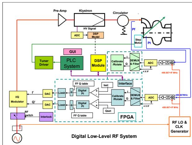
Figure 3: Function blocks of digital low level RF system.
