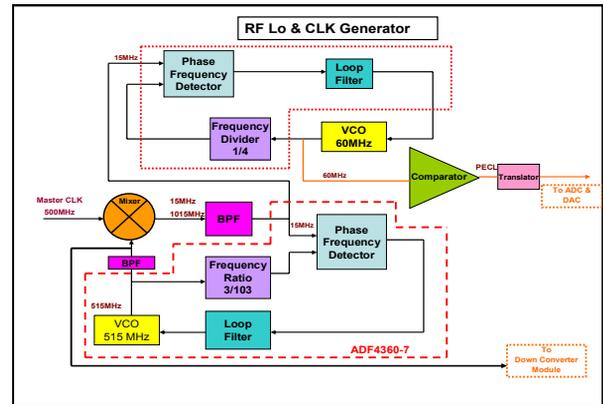
Figure 4: Block diagram of RF LO & Clock generator.
