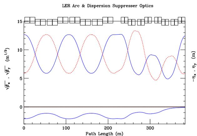
Figure 1: Optics in the arc cells and transition through a dispersion suppresser unit. (Dashed lines are vertical values; solid lines, horizontal). With  $90^\circ$  of phase advance per cell,  $\beta(\max) = 160$  m, and  $\eta(\max) = 2.09$  m.
