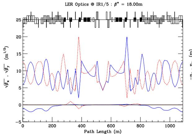
Figure 2: The high luminosity straights IR1 & IR5 with injection optics:  $\beta^* = 18$  m, and  $\beta(\text{max}) = 400$  m.
