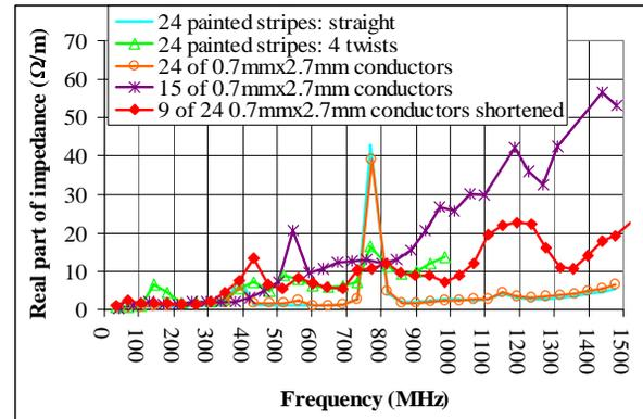
Figure 4: Real part of measured complex impedance, of an LHC injection kicker, for various beam screens.
