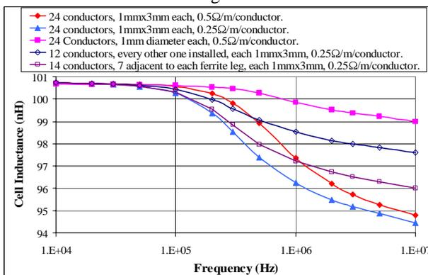
Figure 2: Frequency dependence of the cell inductance for various beam screen conductor configurations.
