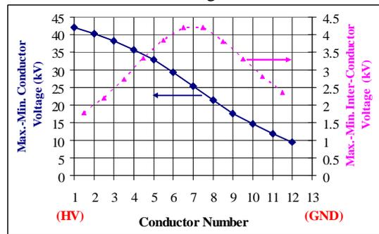
Figure 3: Predicted conductor voltage and inter-conductor voltage for 24 of 0.7 mm x 2.7 mm screen conductors for normal operation at 54 kV PFN voltage.
