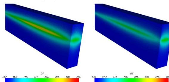
Figure 1.  $\Delta T$  (K) in Ti block 23 for swept bunches at 25 ns intervals (left) and for instantaneous profile (right). The maxima are 401 and 389 K, respectively.
