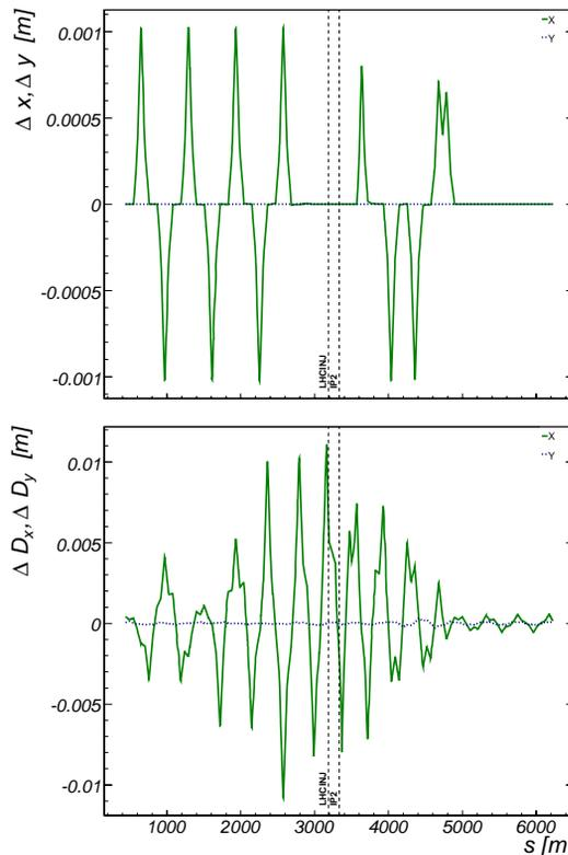
Figure 5: Using resonant orbit bumps: Changes in orbit (top) and resulting dispersion (bottom).
