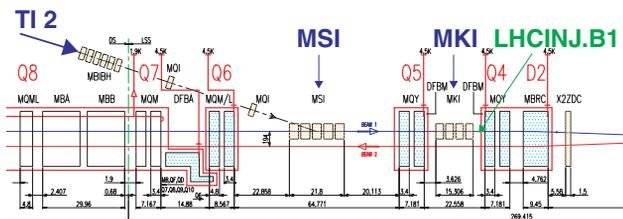
Figure 1: Horizontal view of the IR2 region of the LHC. Beam 1 is injected onto the LHC orbit at the MKI (injection kicker, located between Q5 and Q4) via a *vertical* kick.
