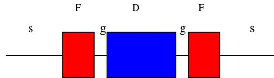
Figure 2: The FDF Triplet Period of each FFAG Ring.
