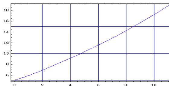
Figure 8: Radial Field Profile of Axial Field in a group of Cavities for FFAG-3 (MV/m vs cm)
