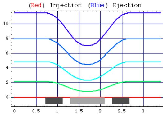
Figure 4: Betatron Tunes during acceleration
