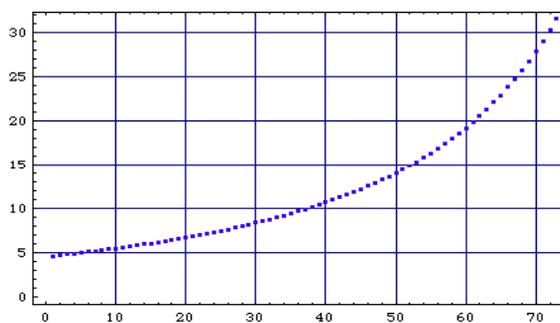
Figure 7: Energy Gain Profile per Cavity Group in FFAG-3 (MeV/u versus no. of crossings)
