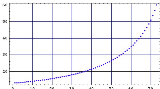
Figure 9: RF Phase Modulation during acceleration cycle (degrees vs. no. of crossings)
