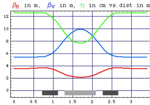
Figure 3: Lattice Functions along a Period at Injection (left) and Extraction (right).
