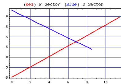
Figure 6: Field Profile (kG vs. cm) of the Sector Magnets in the three FFAG Rings.
