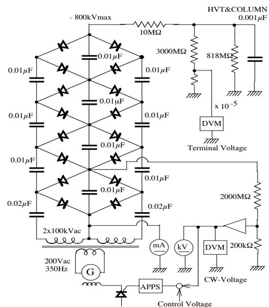
Figure 1: Circuit diagram of the 750keV Cockcroft-Walton high voltage generator..
