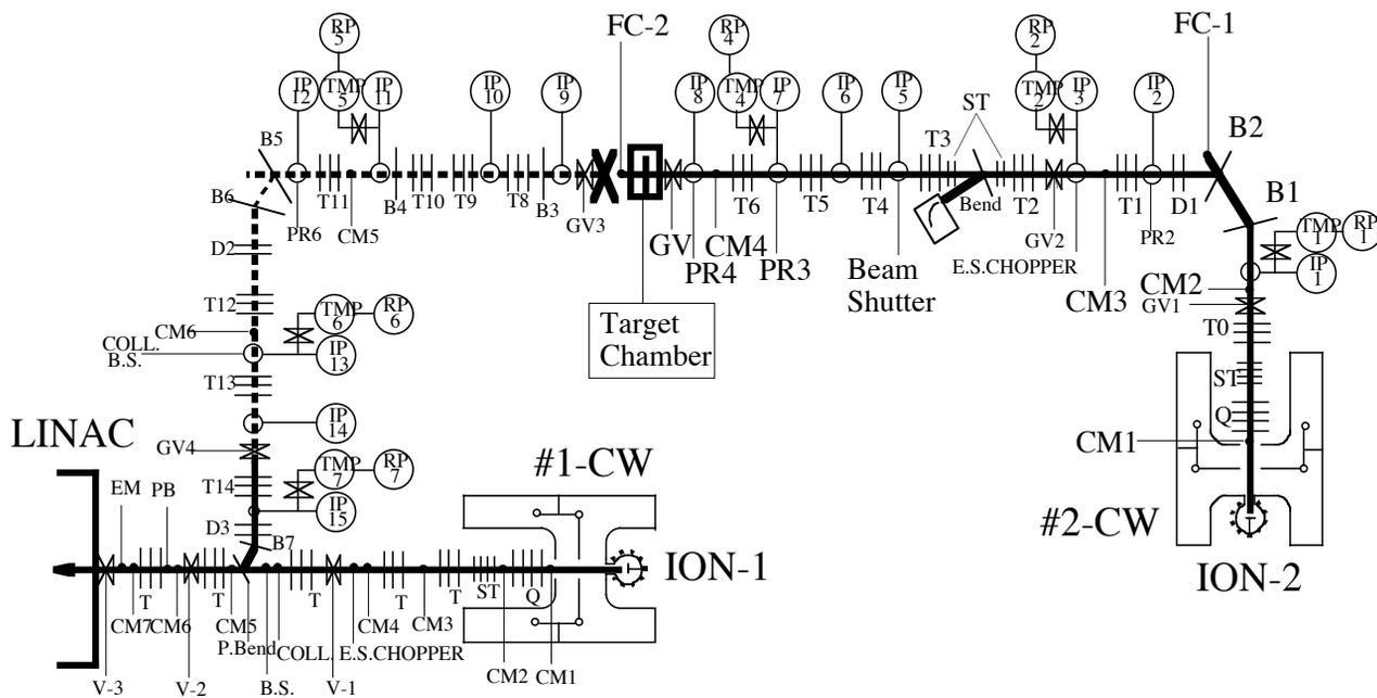
Figure 2: Layout of the low energy beam line for the 750keV pre-injector at 12GeV-
