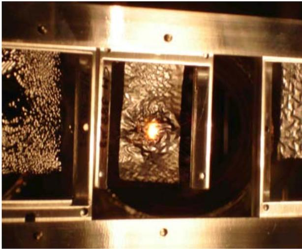
Figure 5: An example of beam spot on the carbon foil.
