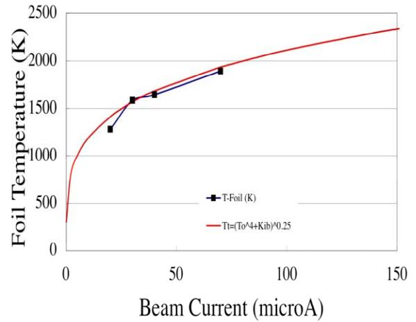
Figure 6: Foil temperature v. s, dc beam current
