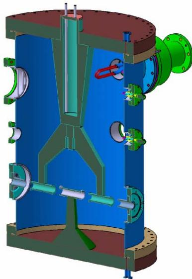
Figure 3: Cross-sectional view of the 4-gap 108 MHz  $\lambda/4$ -resonator buncher cavity.
