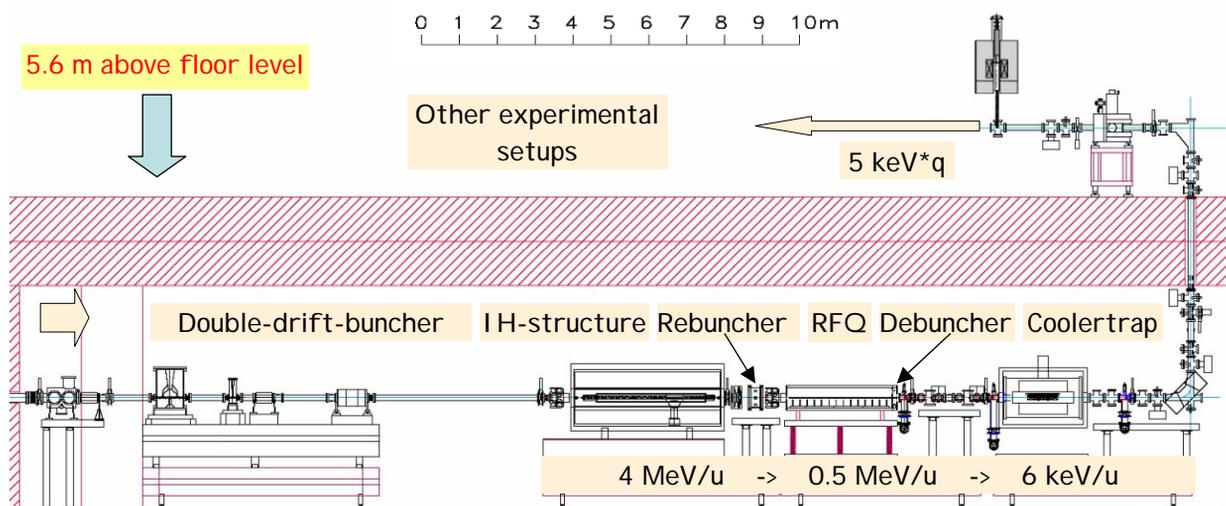
Figure 2: Overview of the HITRAP-decelerator in the reinjection channel.
