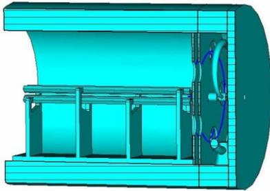
Figure 5: Cross-sectional view showing the low energy end of the RFQ with the integrated debuncher section.
