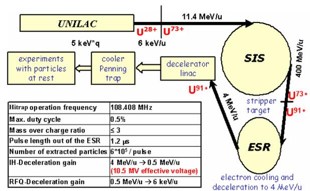
Figure 1: Scheme of the GSI accelerator facility and production process of  $U^{92+}$ .
