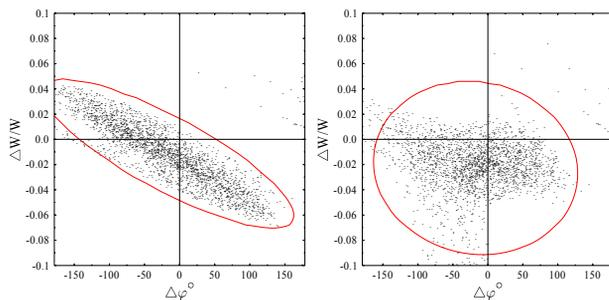
Figure 6: Longitudinal particle distribution at the HITRAP low energy end without (left) and with debunching (right).
