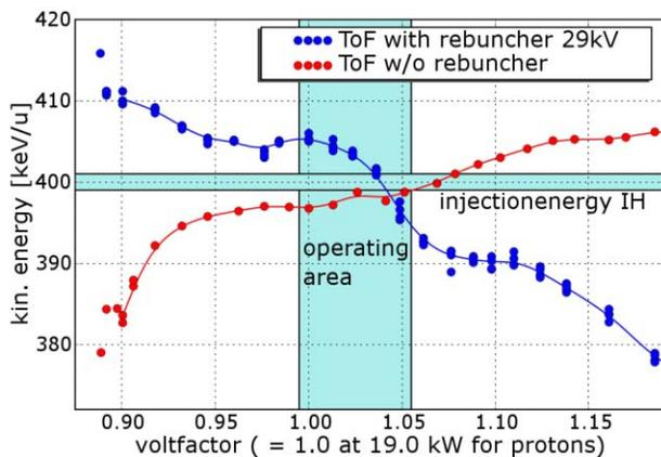
Figure 10: Beam energies behind the RFQ measured at the RFQ test bench at GSI vs. the RFQ voltage factor.
