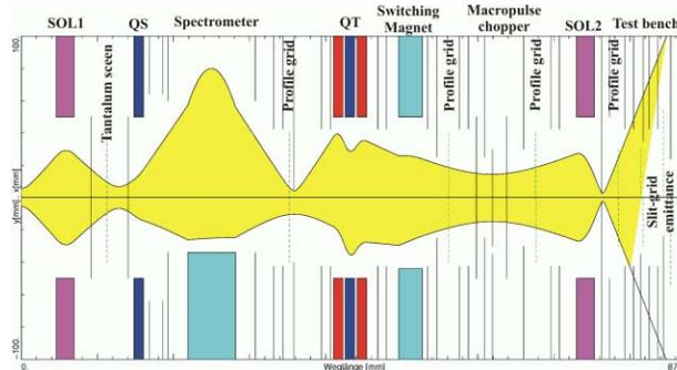
Figure 3: Beam envelopes along the LEBT and the beam diagnostics test bench as calculated with MIRKO [7]. The final solenoid magnet is adjusted to the RFQ.
