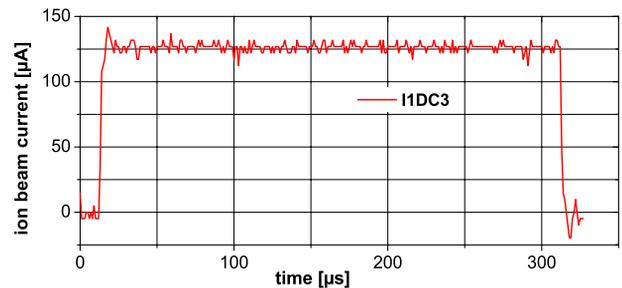
Figure 7: A triggered Faraday cup signal behind the macropuls chopper.
