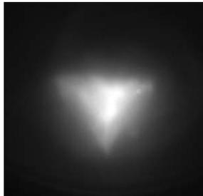
Figure 4: An image of a  $^4\text{He}^{2+}$  beam measured with the tantalum screen behind SOL1.
