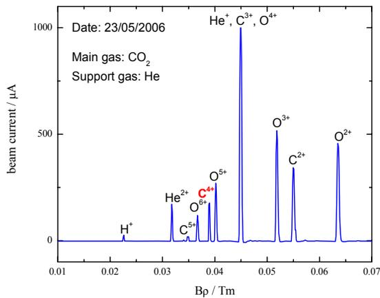
Figure 5: Spectrum of one of the ECR sources. The peak at  $B_p = 0.0386$  Tm corresponds to the desired  $^{12}\text{C}^{4+}$ .
