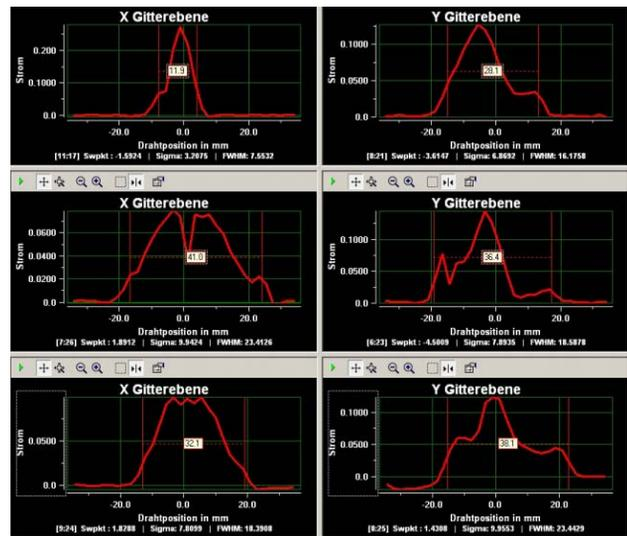
Figure 6: Measured profiles of a  $^4\text{He}^{2+}$  beam along the LEBT. The achieved transmission in this case is 90%.
