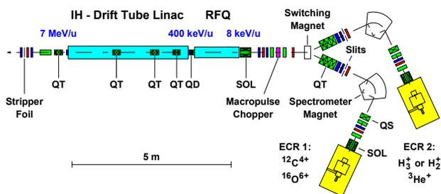
Figure 1: Layout of the Injector Linac [2]. QS = Quadrupole singulet, QT = Quadrupole triplet, SOL = solenoid, magnetic focusing and steering magnets (green), profile grids and the tantalum screen (red), and the beam current monitors (blue).
