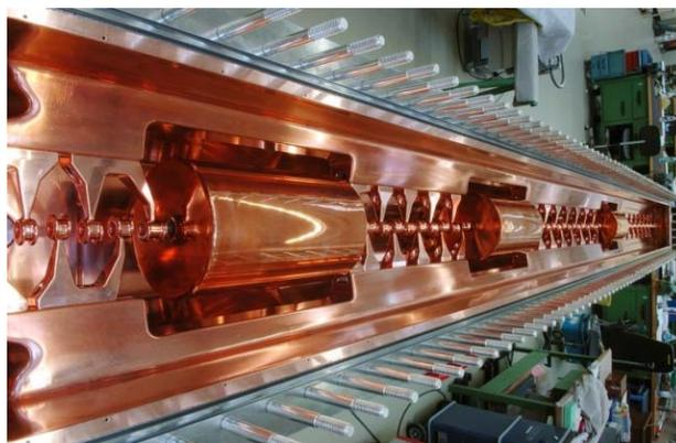
Figure 11: Open IH cavity after copper plating and installation of the drift tubes.
