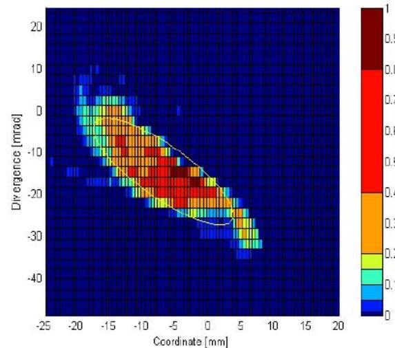
Figure 8: Example of a vertical emittance of a  $200 \mu\text{A}$   $^4\text{He}^{2+}$  beam measured 0.7 m behind the RFQ matching point. The ellipse surface corresponds to a  $4 \times \text{rms}$  emittance of  $80 \pi$  mm mrad.
