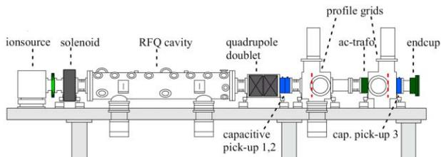
Figure 9: RFQ beam test bench at GSI.
