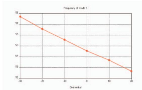
Figure 13: Simulation of the frequency tuning.
