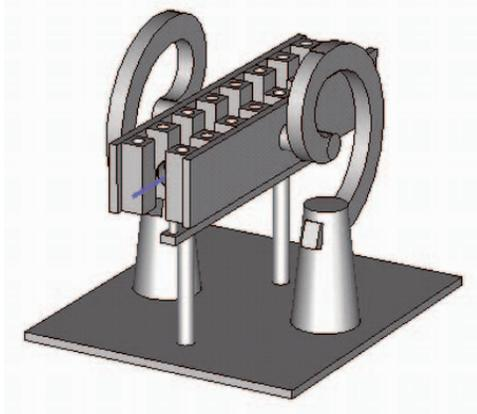
Figure 10: Simulation of the new 15 cell funneling deflector.
