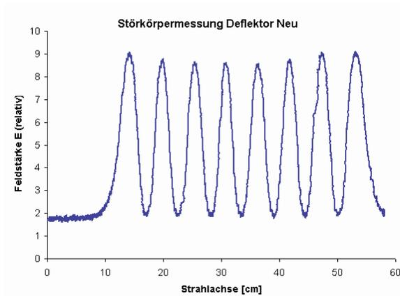
Figure 8: Measured E-field along the beam axis.
