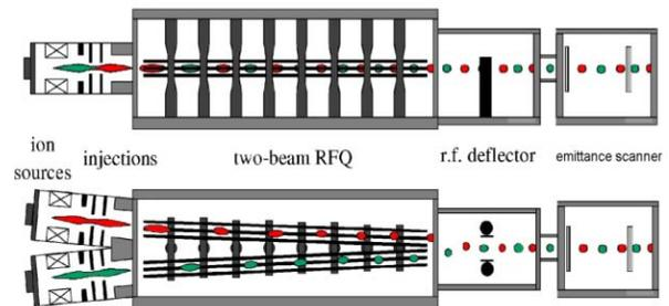
Figure 2: Scheme of the experimental setup.
