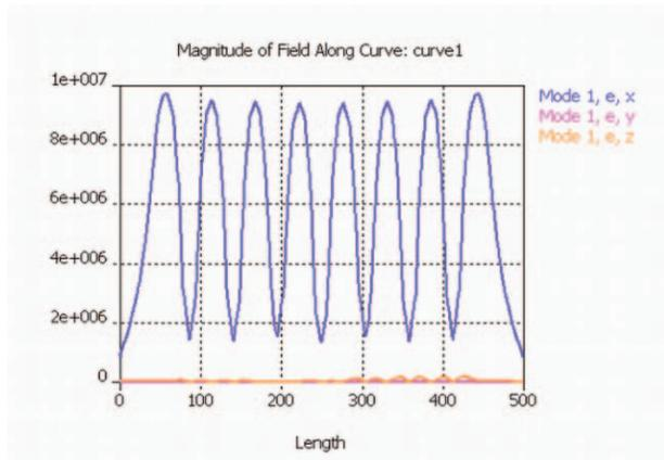
Figure 11: Simulated E-field along the beam axis.
