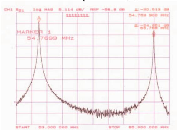
Figure 5: Measured resonance frequencies of the deflector.
