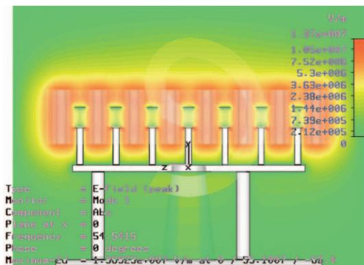
Figure 12: Simulated E-field around the structure.
