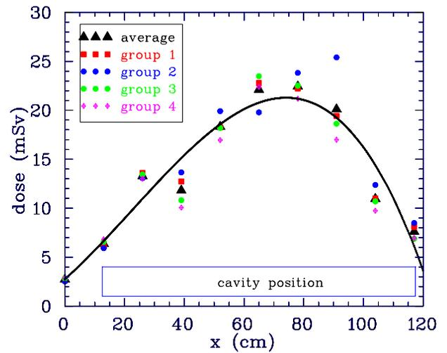
Figure 8: Measured X-ray distribution along the cavity.
