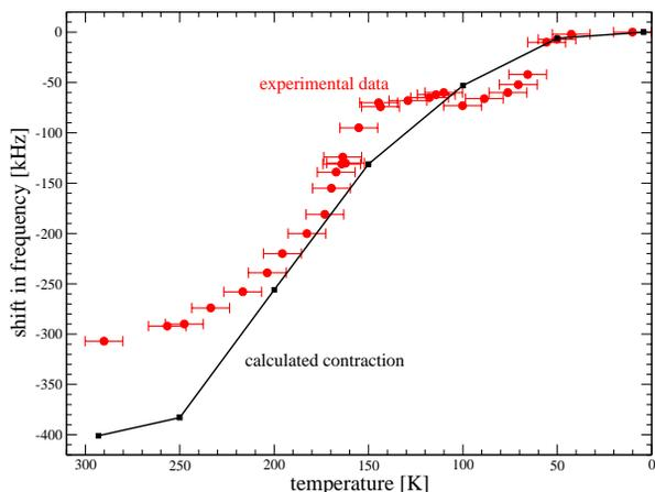
Figure 3: Measured frequency shift during the cooldown. The solid line represents the simulated frequency shift due to the contraction of the material.
