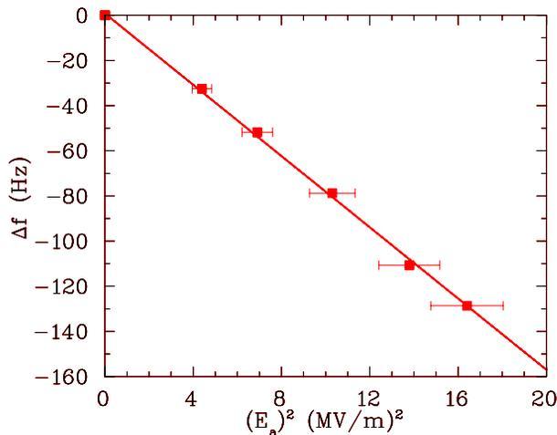
Figure 7: Measured Frequency shift due to Lorentz Force Detuning. The gradient is based on the  $\beta\lambda$ -definition.
