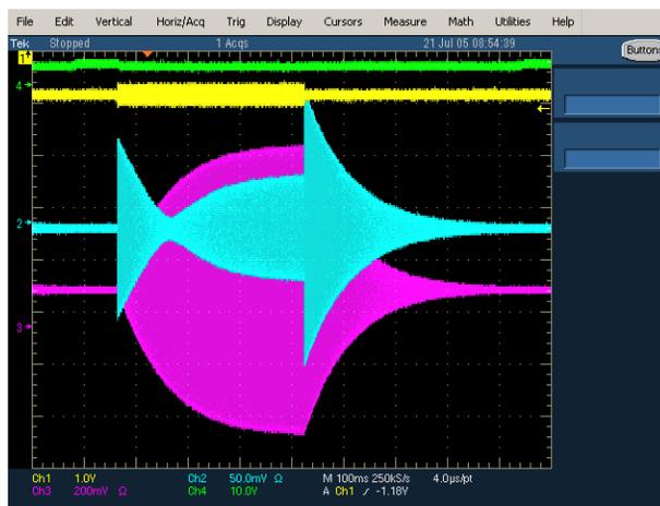
Figure 5: RF signals of the CH-cavity at low fields: Reflected signal (green), pickup signal (magenta) and forwarded signal (yellow). The time scale is 100 ms per division.
