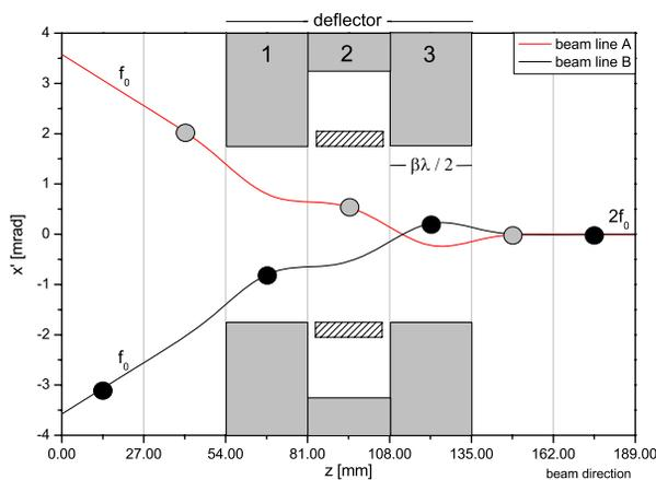
Figure 1: Schematic procedure of funneling.
