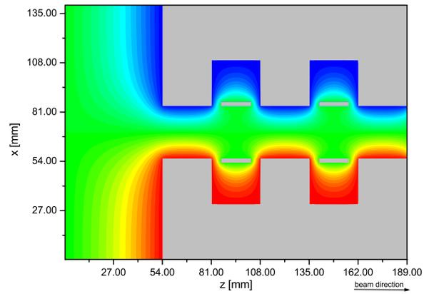
Figure 3: Potential distribution in the first cells of a 15 cell deflector.
