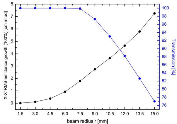
Figure 4: X-X' RMS emittance growth and transmission as a function of the beam radius.
