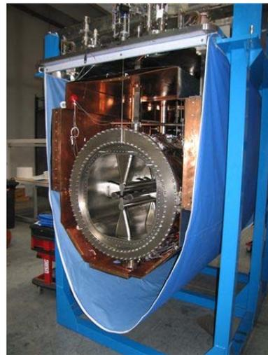
Figure 1: SRFQ resonators in their cryostat.
