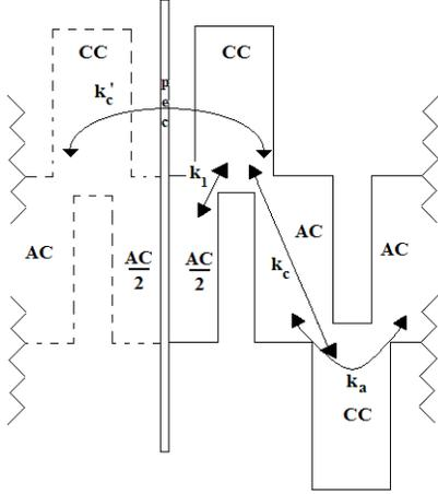
Figure 1: SCL formed by coupling cavities off axis with alternating offset.
